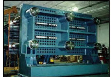
2,500 Ton structural foam injection molding press. Installation was accomplished in 2 hours using hand tools!
