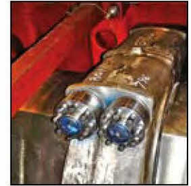
Original nuts were replaced with Superbolt® Torquenuts® on this connecting rod. Accurate preload was achieved quickly with a 3/8" torquewrench, increasing worker safety.
