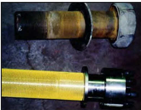
Original bolt (top) and replacement Torquebolt (bottom).
